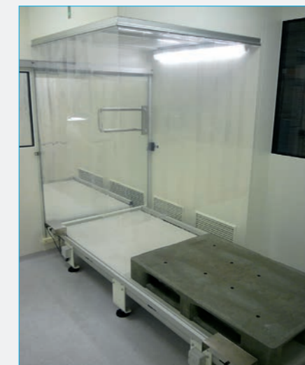
Sampling chamber with laminar flow and conveying technology
