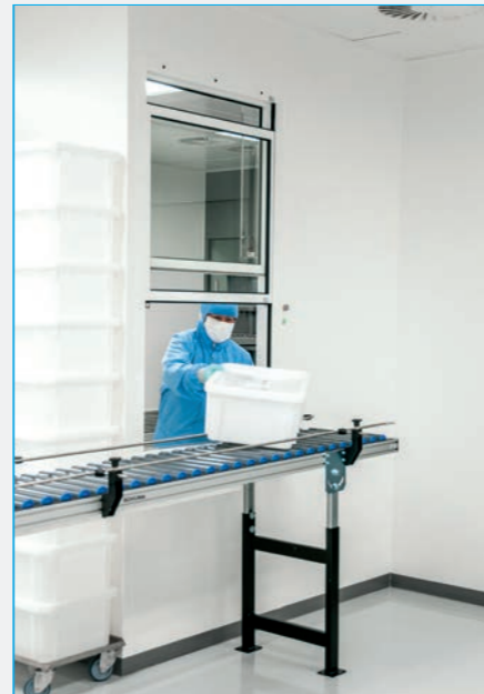
Material air lock with ultrasonic cleaning system
